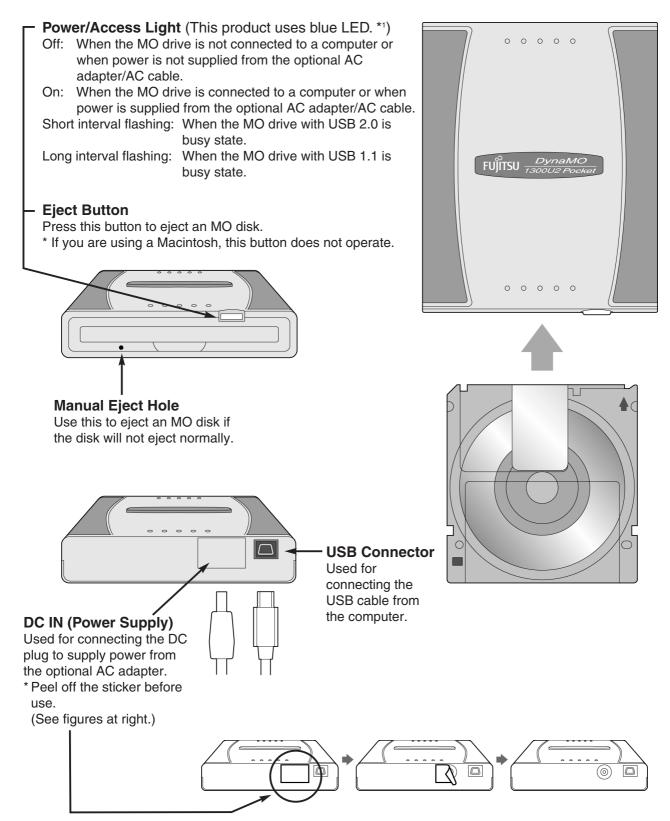
\*1 According to International Electrotechnical Commission provides standard IEC60073 and IEC60204-1 "The meaning concerning the state of the color of the display light and the machine", a blue display light has an obligatory meaning (The state to demand the behavior of those who operate it is indicated). This product adopts blue LED by occasion of the design. There is no meaning about the LED color that the behavior of those who operate it is demanded.
