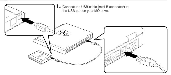
**2.** Connect the USB cable (A-type connector) to the USB port on your computer.
